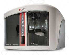
Beckman Coulter Counter for determining of cell volume, particle number, mass and surface area size distributions from one measurement
