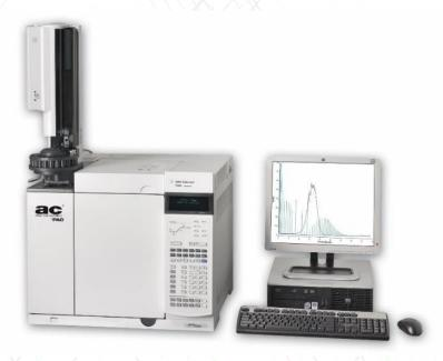
The AC Simulated Distillation (SIMDIS) applications use gas chromatographic (GC) analysis to determine true boiling point distribution up to 750°C of crude oil and crude oil fractions
