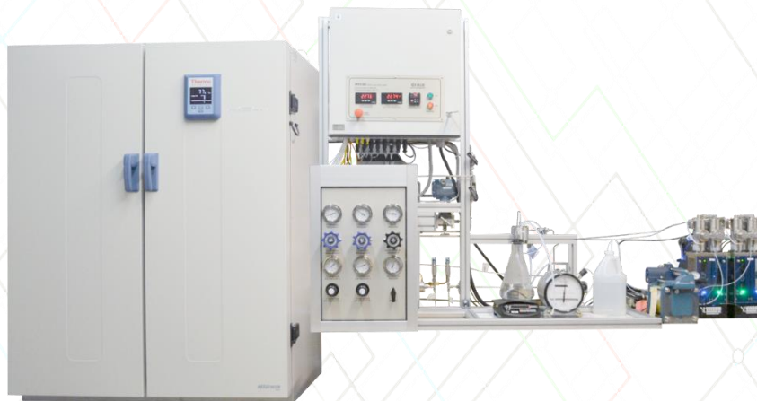
Core Analysis Instruments - measure shale reservoir rock properties such as permeability, porosity and saturation.
