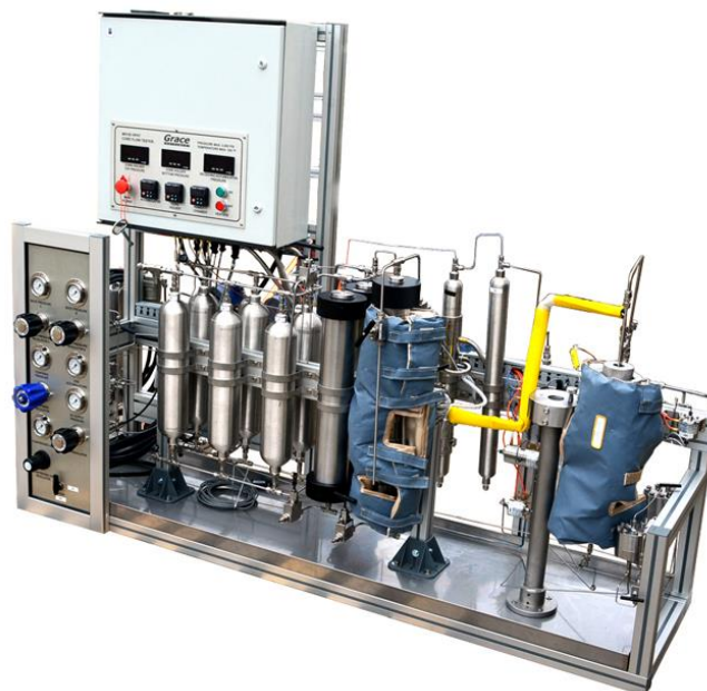
Core Analysis Instruments - measure shale reservoir rock properties such as permeability, porosity and saturation.
