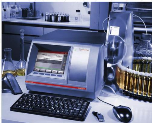
**Densimètre automatique digital** conforme aux normes ASTM D 1250, ASTM D 4052, ASTM D 5002, ASTM D 5931 ANTON PAAR
